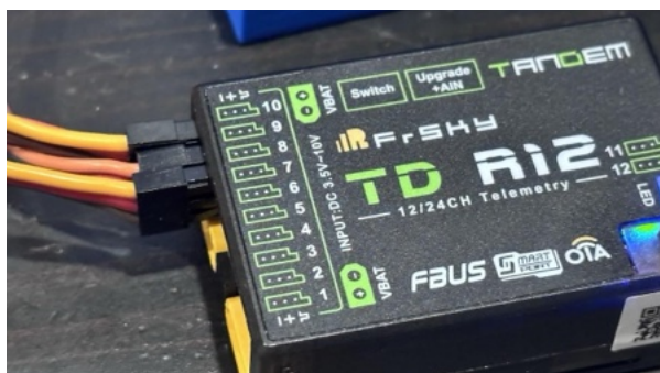
Multiple types of sensors plugged individually into ports 10/8 of TD R12
