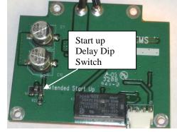
Glow drivers shipping after Sept 2008 now have the ability for the user to turn on or off a start-up delay feature commonly used for pattern flying). To set the delay, remove the four screws on the back side of the case, and locate the dip switch on the back side of the board.
